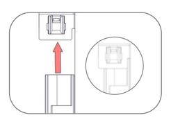
**6.** Slide the side extrusion up until its slots into the top corner fixing bracket. The side extrusion should rest under the bracket.
