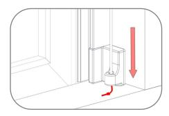
**12.** If your blind requires further tension pull the cord through the hole in bottom button until you feel the blind has sufficient tension and tie a fresh knot.
