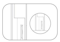
**8.** Push the slot at the base of the extrusion over the bottom corner bracket. Gently push the extrusion against the glass to ensure tape has adhered. Repeat for both sides.
