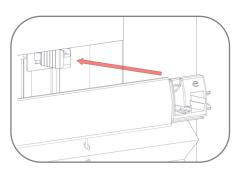
**9.** Align headrail endcaps with top corner fixing brackets and push fully home.
