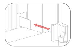
**10.** Align bottom button with bottom corner brackets. Slide the bottom button onto the bracket until it locates. Repeat both sides.
