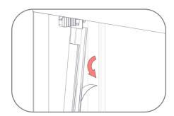
**7.** Pivot the extrusion towards yourself so you have access to the back. Peel the backing from the glass tape and slowly place the extrusion against the glass.
